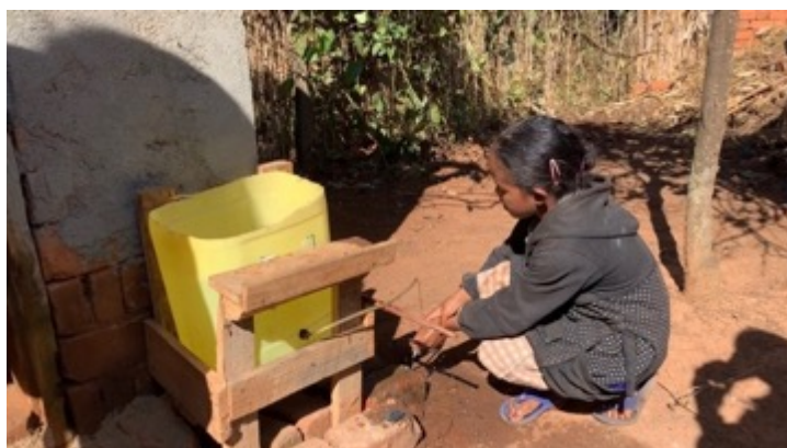
One of the handwashing stations made from a jerry can, tubing, and wooden frame. The tubing sits vertically in a wooden notch when not in use to stop water flow. (photo credit RANO WASH)
