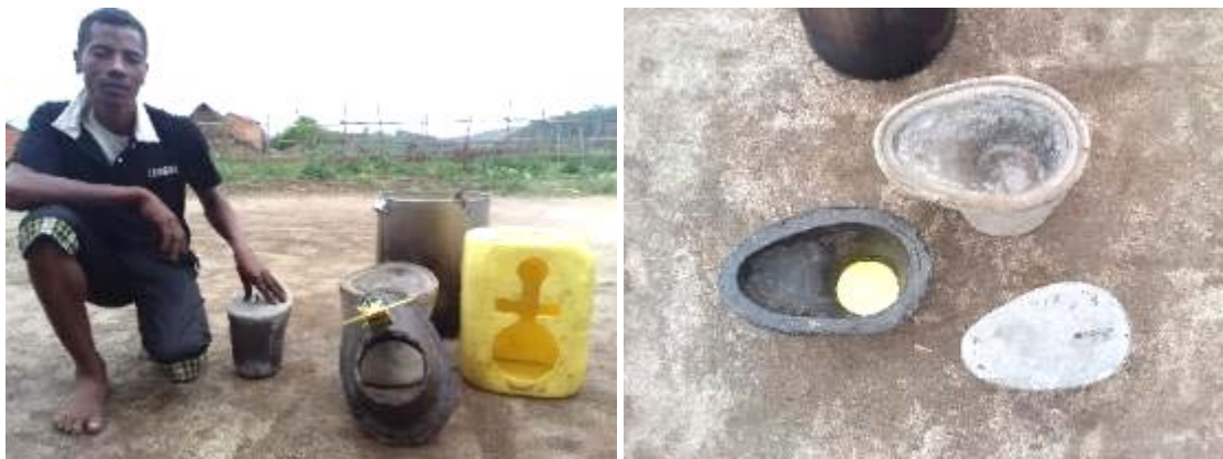
Picture 2: Toilet seat and lid with ferrocement and washable tile with plastic waste recycled by a local mason, Ramanadafy Heritiana, in Vodiriana, Alaotra Mangoro
