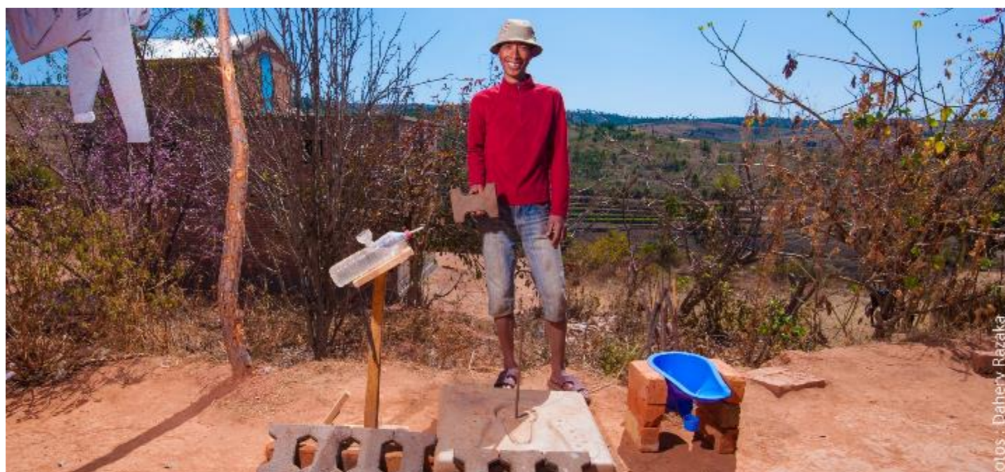
Emmanuel, a local mason from Ambohitsimanova, Vakinankaratra region has invented a responsible and anti-pollution formula. These bricks are made from sand and plastic waste to build and decorate the latrines of his clients.
