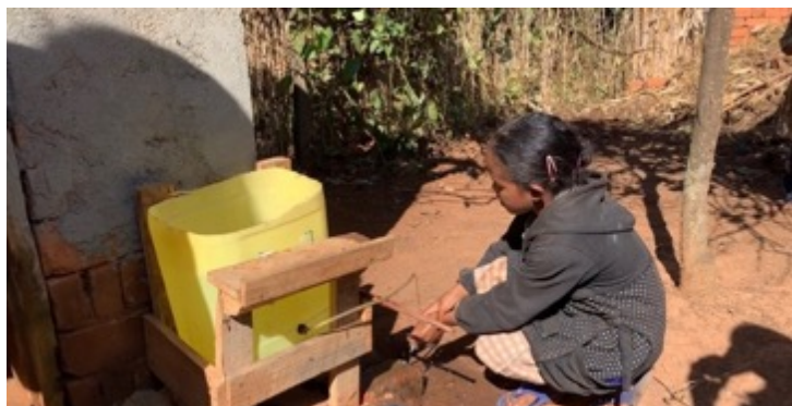
One of the handwashing stations made from a jerry can, tubing, and wooden frame. The tubing sits vertically in a wooden notch when not in use to stop water flow. (photo credit RANO WASH)
